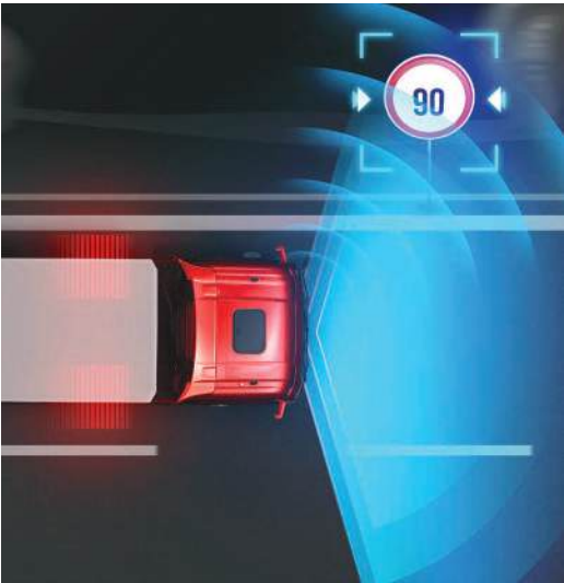
ISA - TRAFFIC SIGN RECOGNITION Recognizes speed limits using camera and navigation data, warns in case of violations, and intervenes when necessary.
